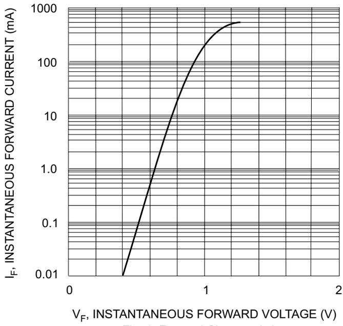
Fig. 1 Forward Characteristics
