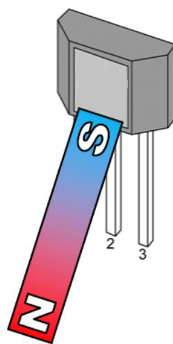
$V_{OUT} = 2.5 \text{ to } 4 \text{ V}$
