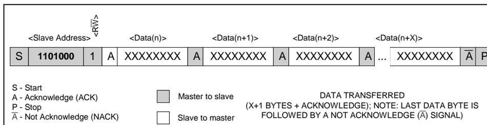
**Figure 6. Data Read (Write Pointer, Then Read)—Slave Receive and Transmit**
